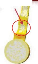
Figure 6 – The arrow points to cavitation caused by a sharp turn in a sprue.
