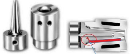
Figure 1 - A drip that gets "pinched" between the sprue bushing and the sprue post can crack the post and allow water to enter the nozzle and gooseneck!
