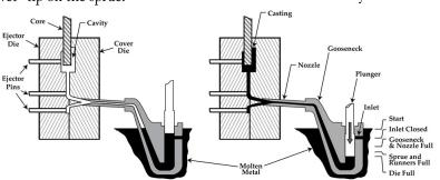
Figure 2 – Clearing the nozzle of molten metal must happen each and every cycle. Set the die slightly above the platen centerline in order to create a slight uphill angle in the nozzle. Setting the nozzle at a slight angle will help to accomplish this.
