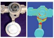
Hydraulic oil filter head, Top Die Casting.
